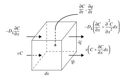
Figure 1.--Terms in the advection-reaction-dispersion equation.
